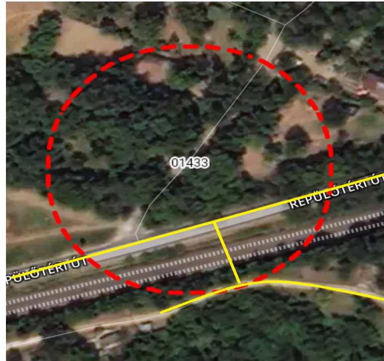
01433 – no access to 200mm pipe, runs under train – recommend further investigation
